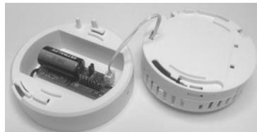
4) Fit all alarms to their own Radio Pattresses by lining up the two arrows as shown below—
