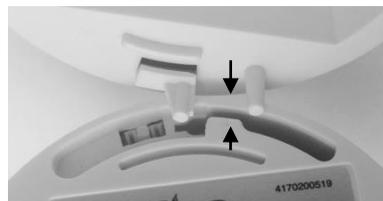
5) Close the alarm onto the Radio Patress and turn the alarm clockwise to lock it into place. This action automatically turns the alarm on.
